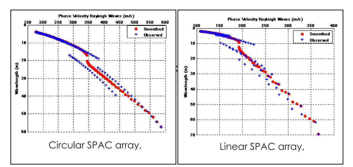
Fig. 3 Results from the inversion of the auto correlation function from which the phase velocity of Rayleigh waves was obtained
