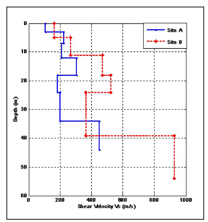
Fig. 5 Obtained shear wave velocity model profiles for sites A and B.
