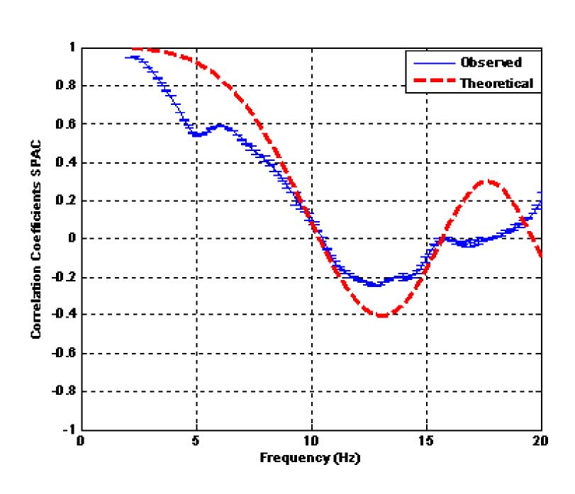
Fig. 2 Autocorrelation coefficients averaged observed and their fit to zero order Bessel function.
